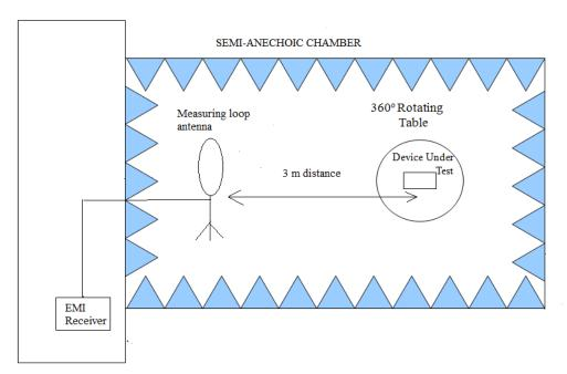
Shielded Control Room For Radiated Measurements
