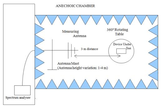
Shielded Control Room For Radiated Measurements
