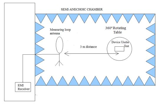
Shielded Control Room For Radiated Measurements
