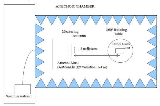
Shielded Control Room For Radiated Measurements
