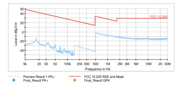
Note: The scan is performed with a peak detector.
