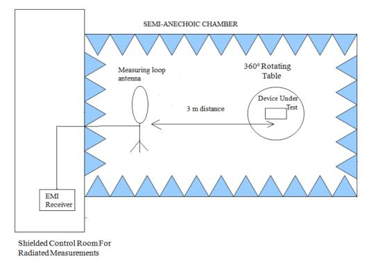
Radiated measurements setup f > 30 MHz up to 200 MHz:
