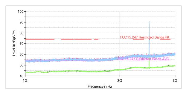
The peak above the highest limit is the Bluetooth LE carrier frequency.
