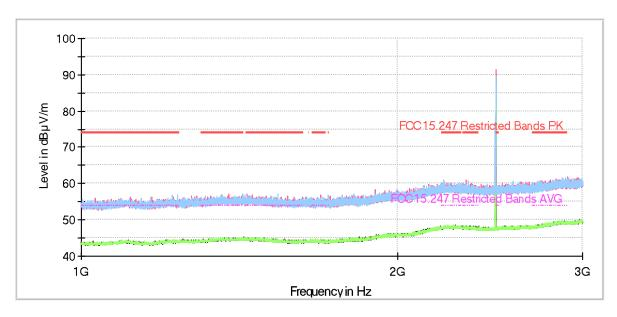
The peak above the highest limit is the Proprietary protocol 2.4 GHz carrier frequency.
