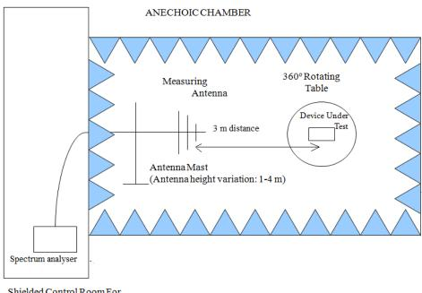
Shielded Control Room For Radiated Measurements
