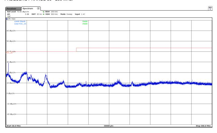
Note: The scan is performed with a peak detector.
