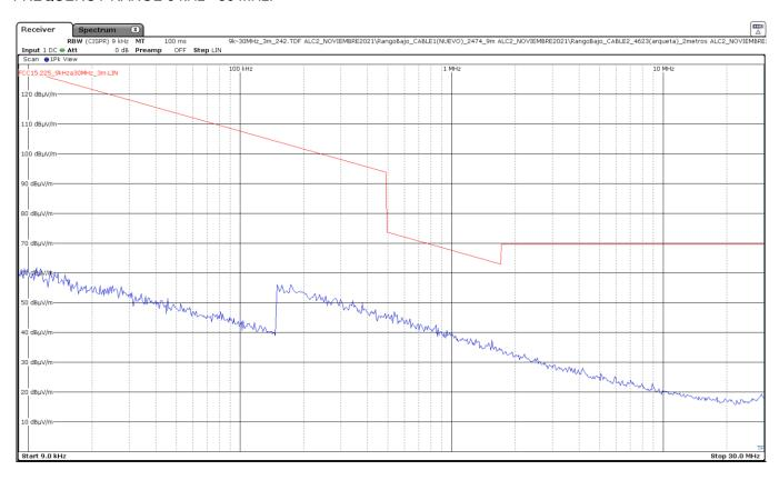
Resolution bandwidth: 200 Hz for 9 kHz  $\leq$  f  $\leq$  150 kHz 9 kHz for 150 kHz  $\leq$  f  $\leq$  30 MHz
