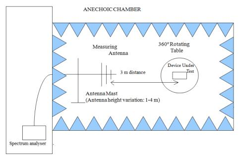
Shielded Control Room For Radiated Measurements
