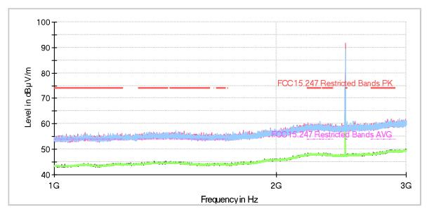
The peak above the highest limit is the Proprietary protocol 2.4 GHz carrier frequency.
