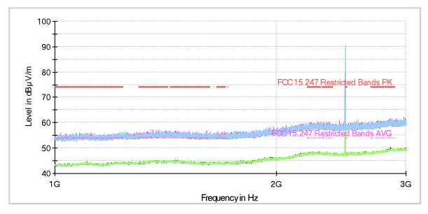
The peak above the highest limit is the Bluetooth LE carrier frequency.
