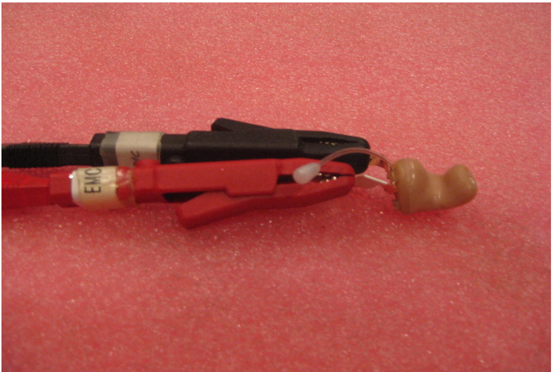
Photo 4.5.2 Test setup regarding measurement of field strength of fundamental.
