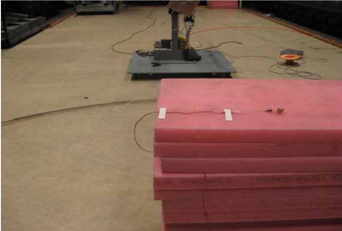
Photo 1.1.7 Test setup regarding measurement of radiated emission, 1 GHz to 25 GHz.
