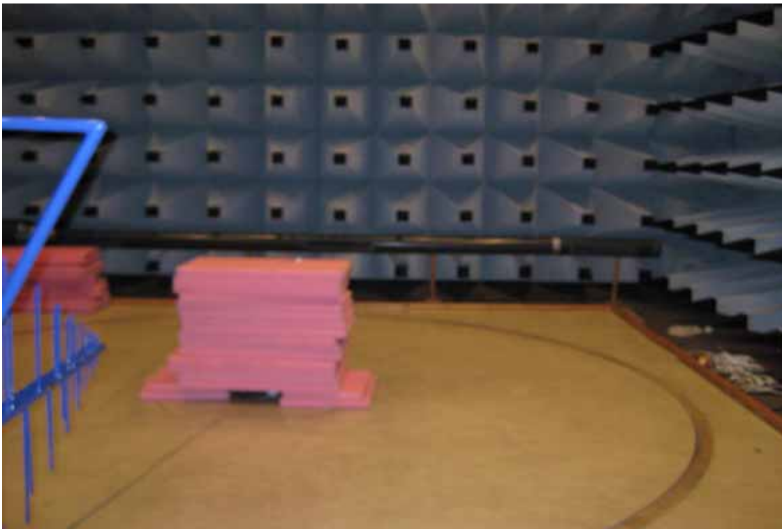
Photo 4.4.4 Test setup regarding measurement of radiated emission, 30 MHz to 1000 MHz.
