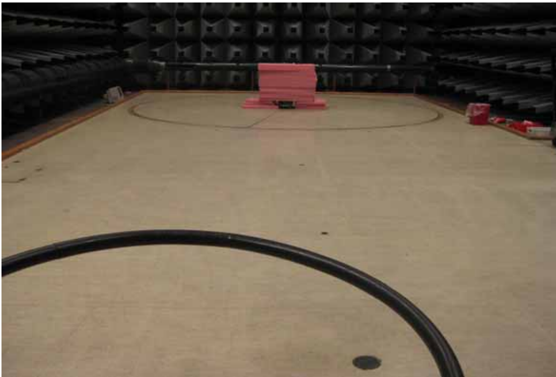
Photo 4.4.2 Test setup regarding measurement of radiated emission, 0.009 MHz - 30 MHz.
