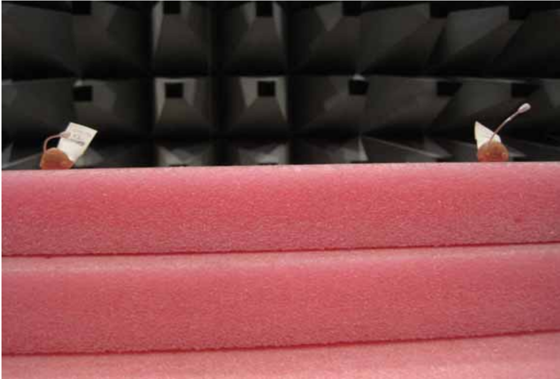
Photo 4.9.3 Test setup regarding measurement of radiated emission, Rx, IC, 1 GHz to 25 GHz.
