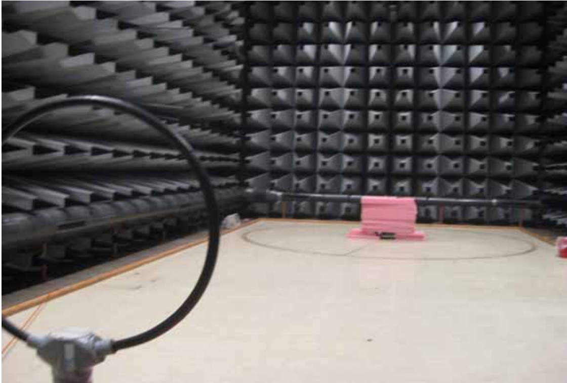
Photo 4.4.1 Test setup regarding measurement of radiated emission, 0.009 MHz - 30 MHz.
