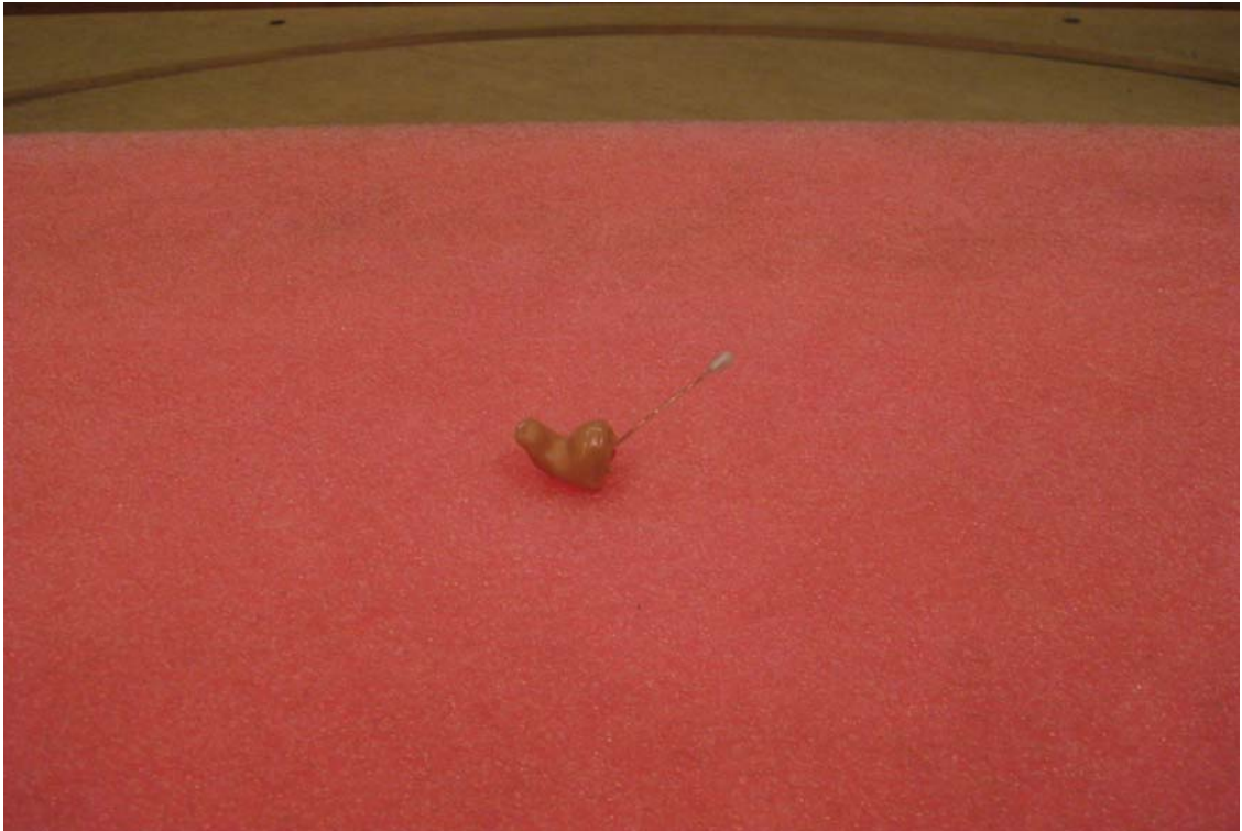
Photo 4.5.2 Test setup regarding measurement of radiated emission, 30 MHz to 1000 MHz.
