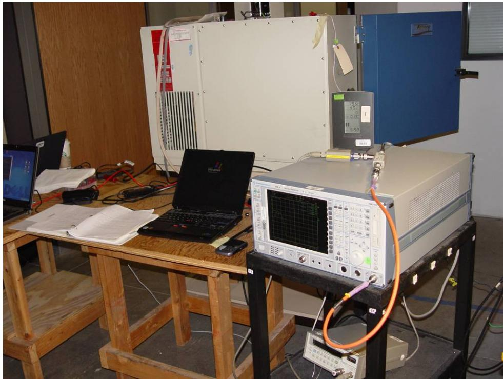
AC Wireline Emissions Test Set-Up
