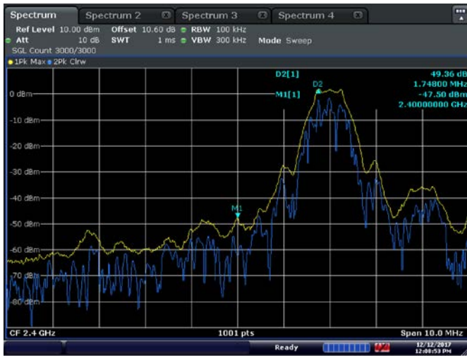
Figure 8.3.1: Band-edge Measurement, low channel
