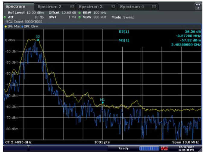
Figure 8.3.2: Band-edge Measurement, high channel
