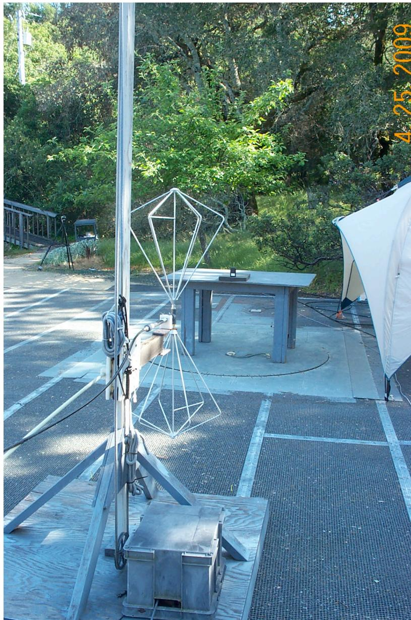
**Front of Radiated Test Configuration, 30 MHz to 1 GHz**
