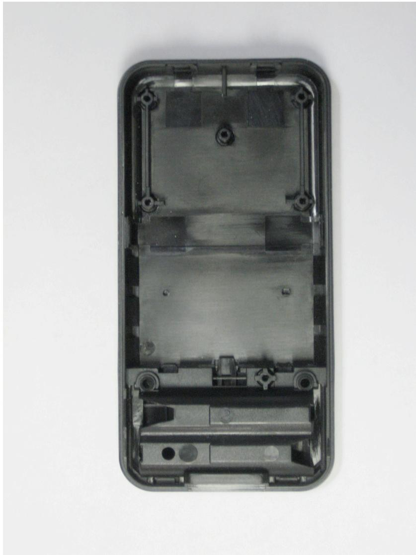
**Inside of front half of non conductive plastic case showing mounting of batteries**
