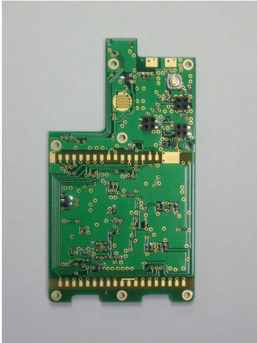
**Backside of Teflon board removed from rear case half**
