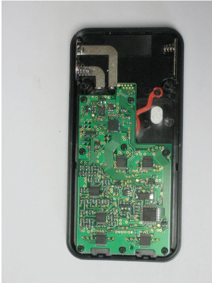
Back side of display board removed from front case half
