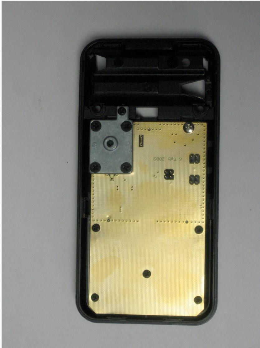
Front side of display board mounted in front case half
