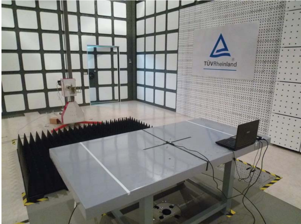
Photograph 4: Set-up for Conducted testing
