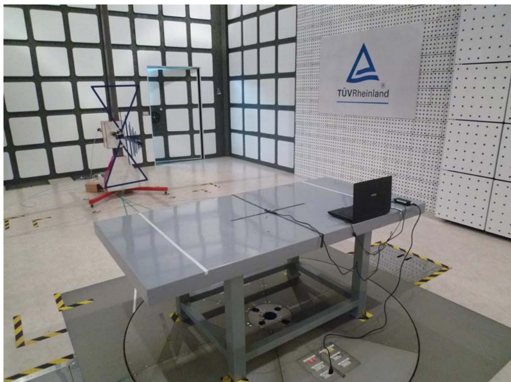
Photograph 2: Set-up for Spurious Emissions (Back View 1)
