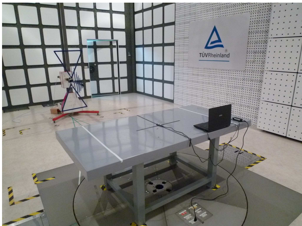
Photograph 2: Set-up for Spurious Emissions (Back View 1)
