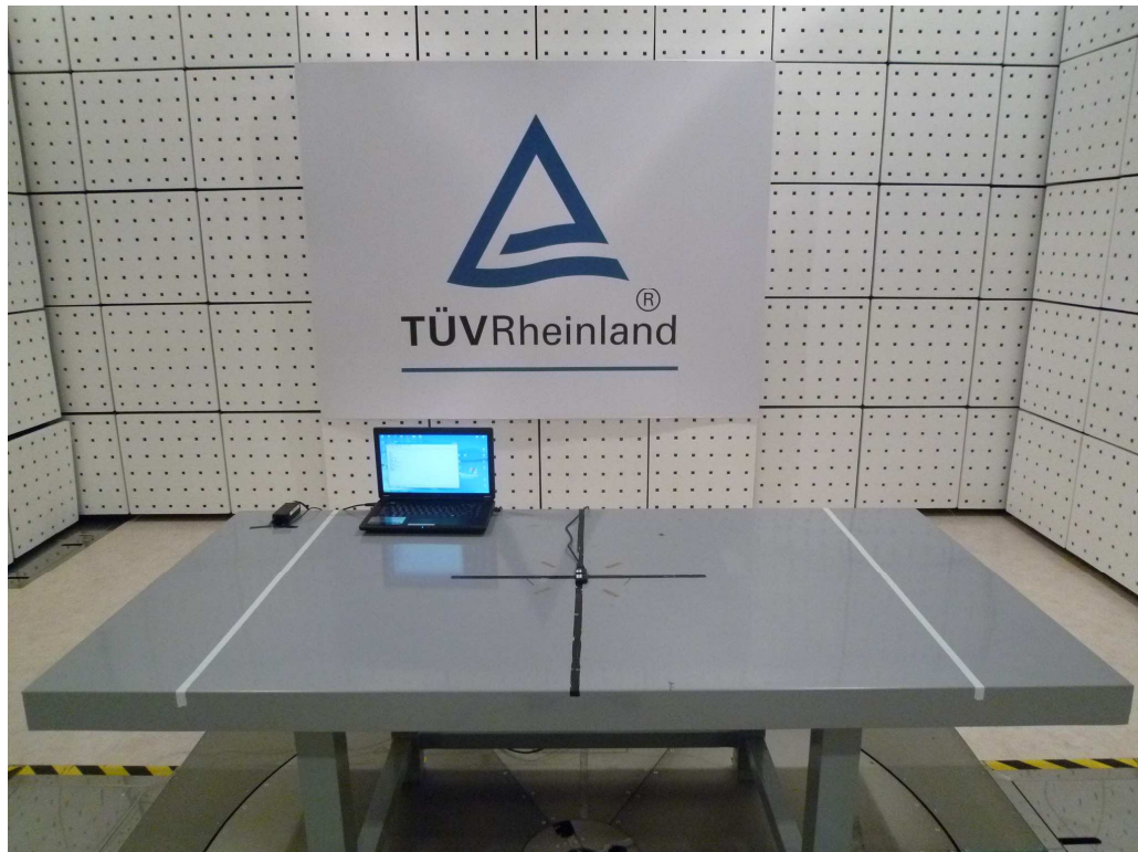
Photograph 2: Set-up for Spurious Emissions (Back View 1)
