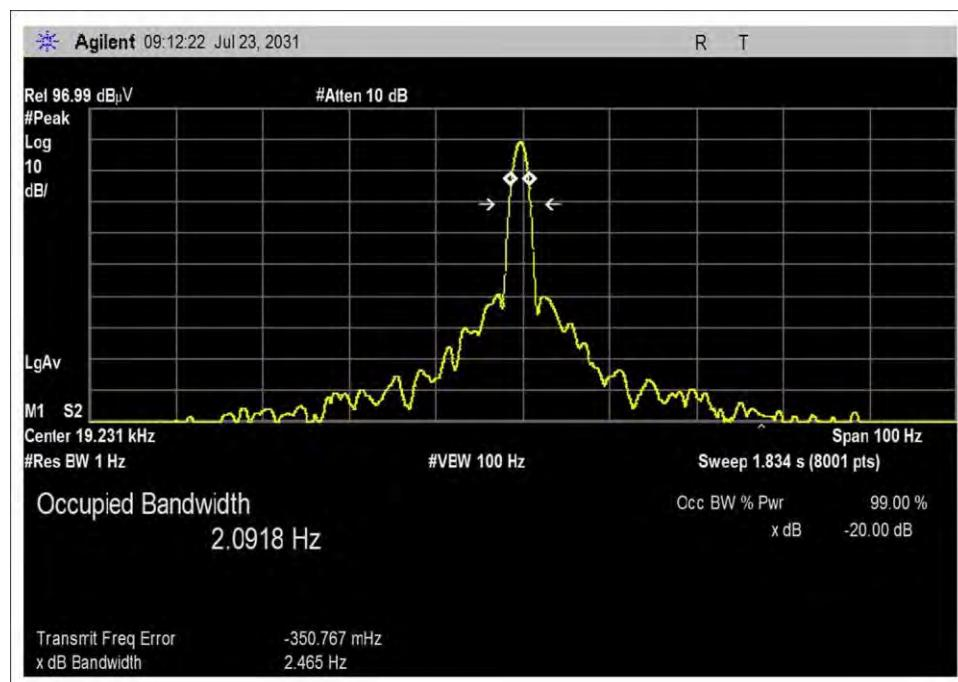
Note: The above time stamp referenced is set at a default setting; the actual test date should read September 19, 2014. The screen capture above was taken at the time of testing and cannot be changed.
