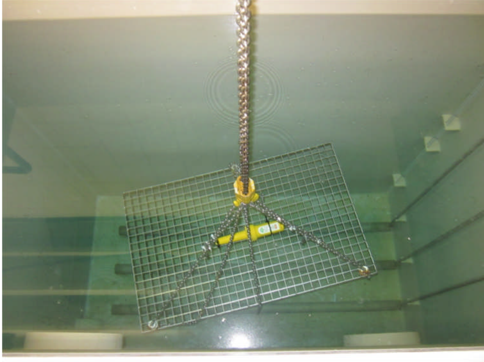
Photo 7: Test set-up, water immersion (temporary immersion)
