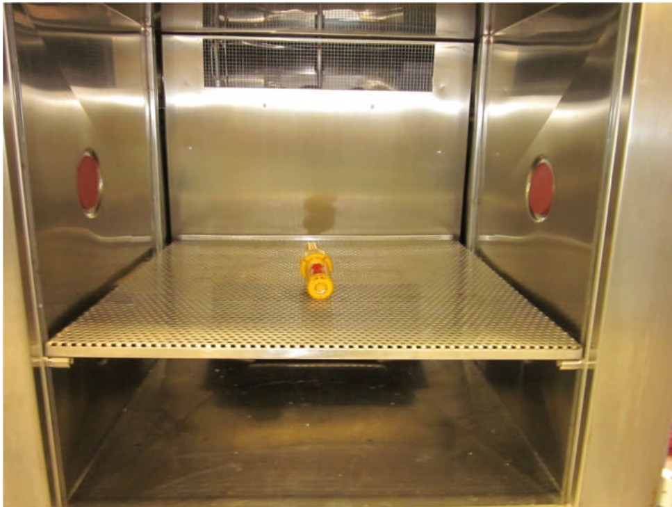
Photo 1: Test set-up EUT in climatic chamber
