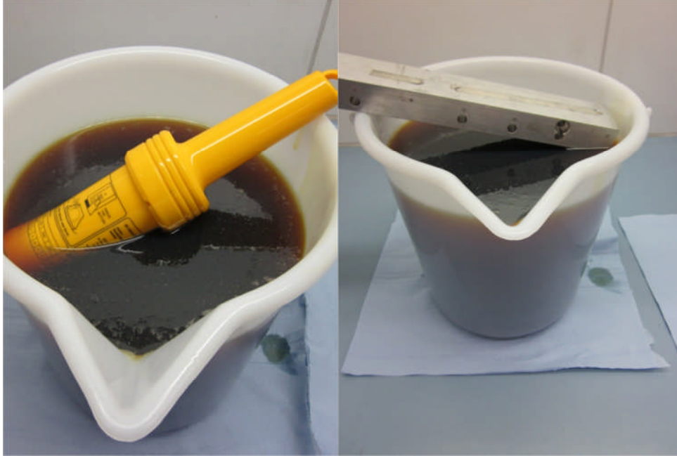
Photo 5: Test set-up, oil resistance (exemplary)
