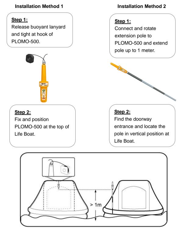
Figure 3-1-3 Mounting process
