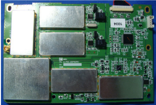
Figure 8: Top View of RF Module
