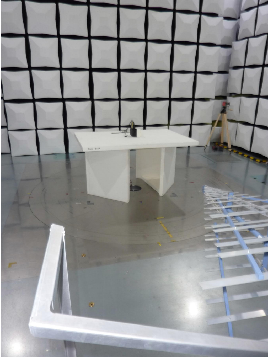
Test setup fully anechoic chamber (below 1 GHz)
