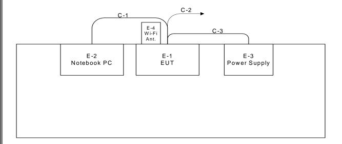
C-1 USB Cable C-2:DATA Cable C-3:DC Power Cable
