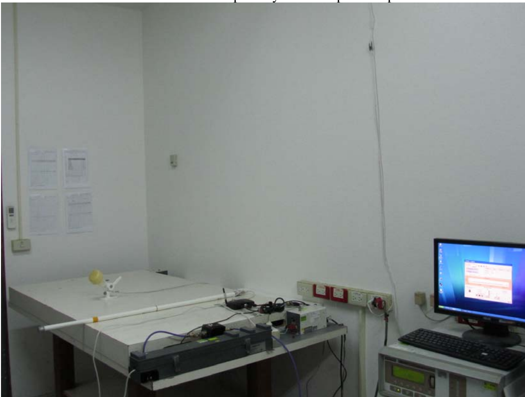
Conducted Susceptibility Test Setup - Clamp
