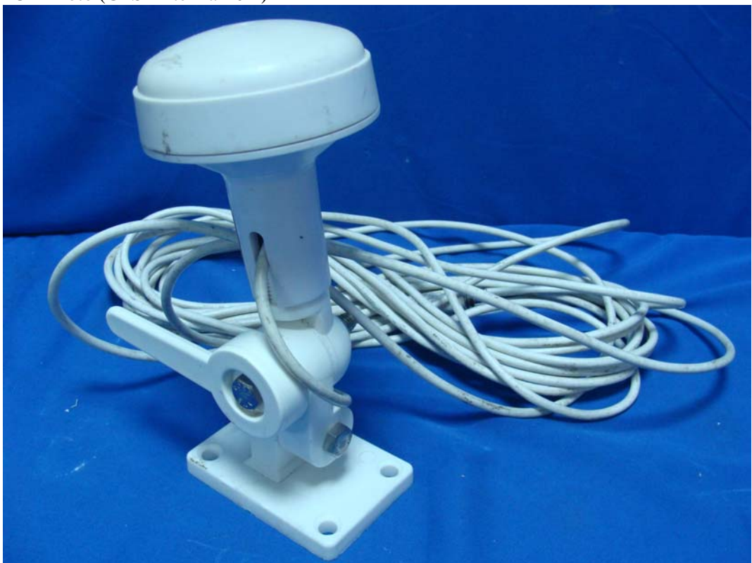
(20) EUT Photo (GPS Antenna-10m)
