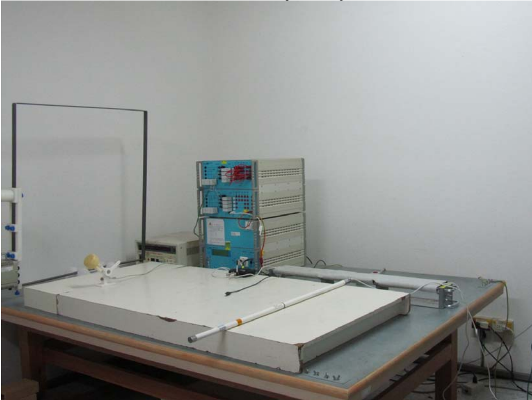
Conducted Susceptibility Test Setup - Clamp
