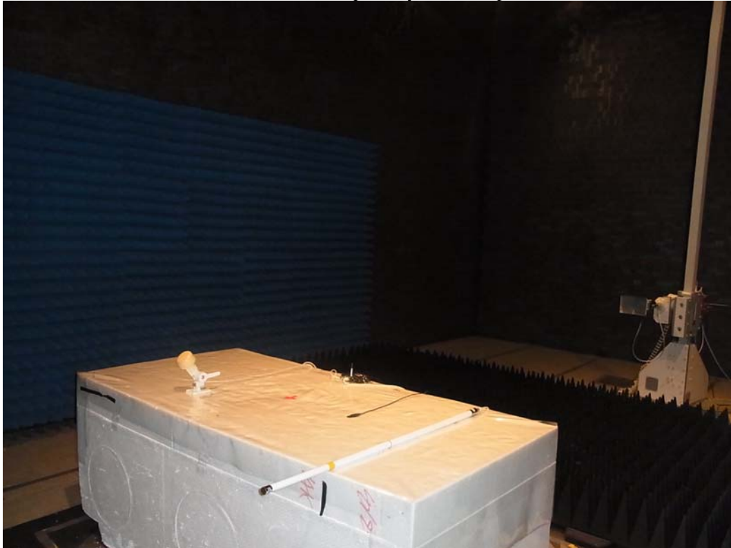
Radiated Susceptibility Test Setup
