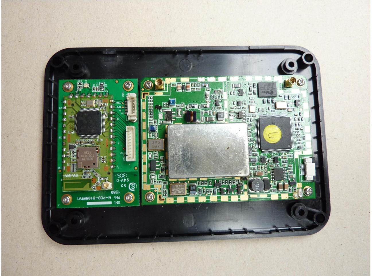
123924eut4.jpg: Main-PCB, front-view
