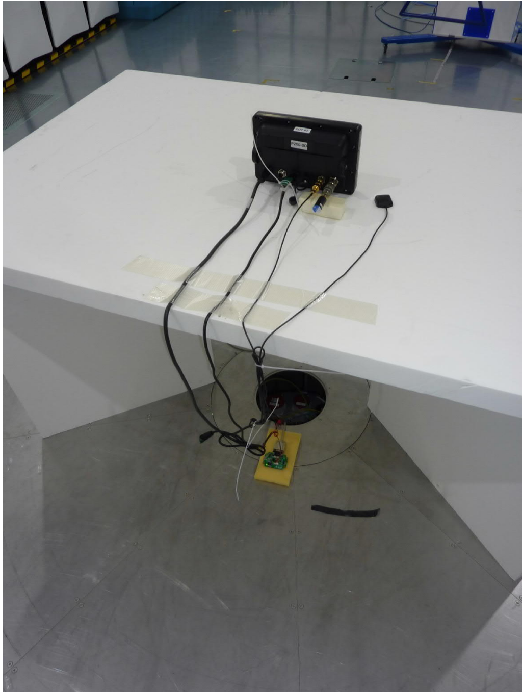
Test setup semi anechoic chamber (position 1)
