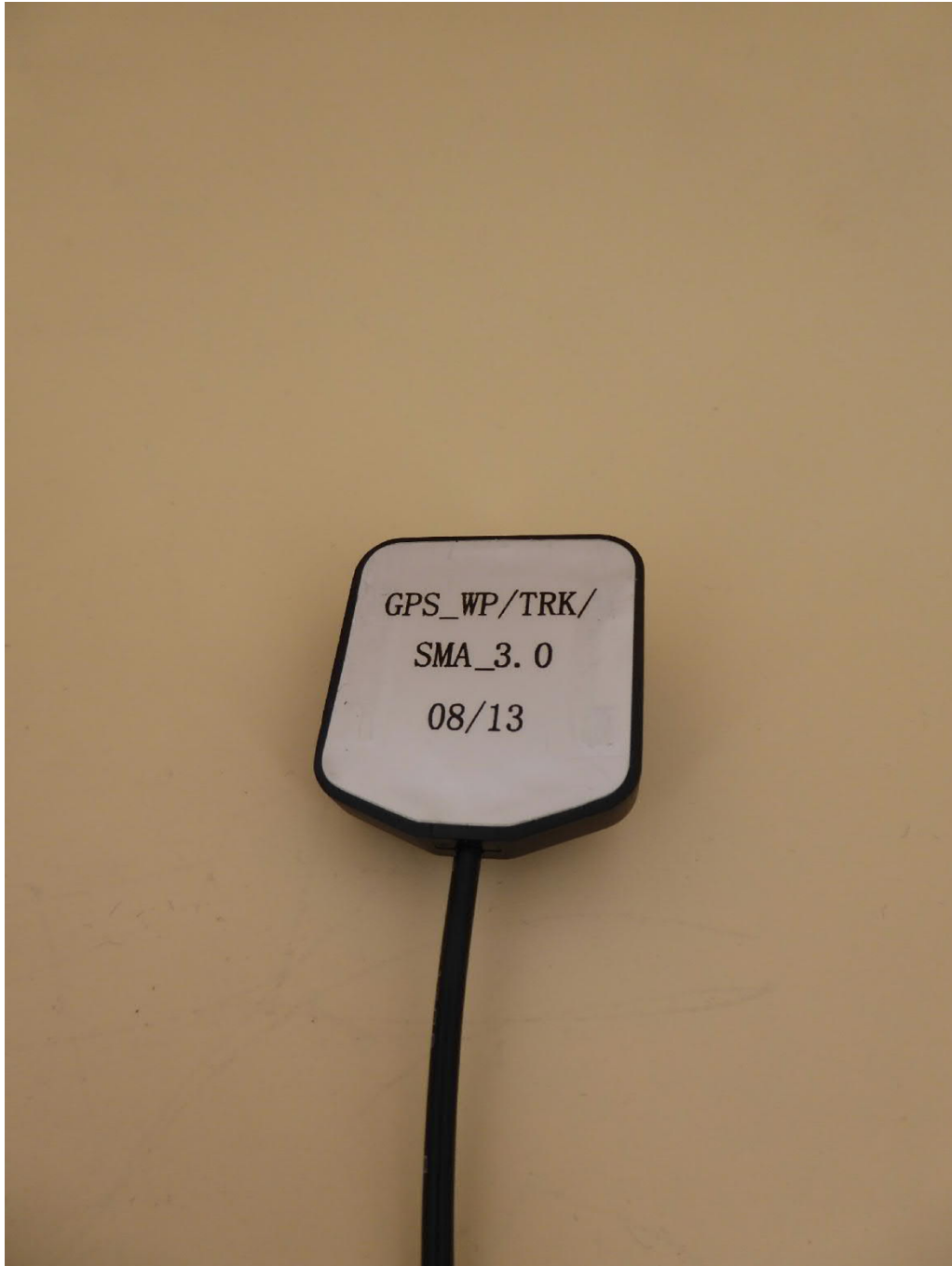
GPS antenna used for radiated tests
