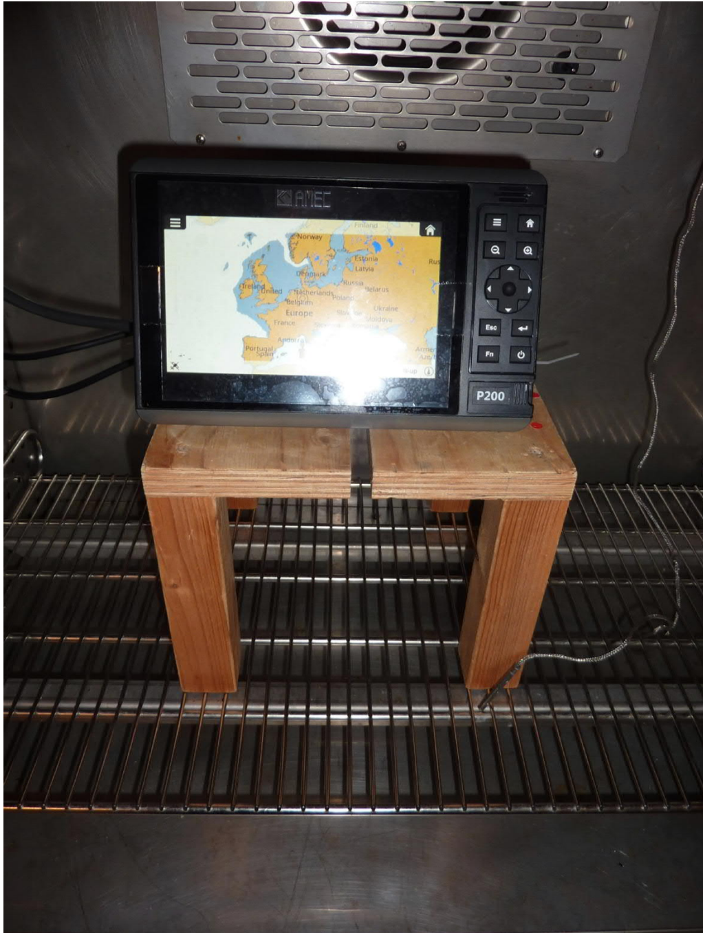
Test setup temperature chamber
