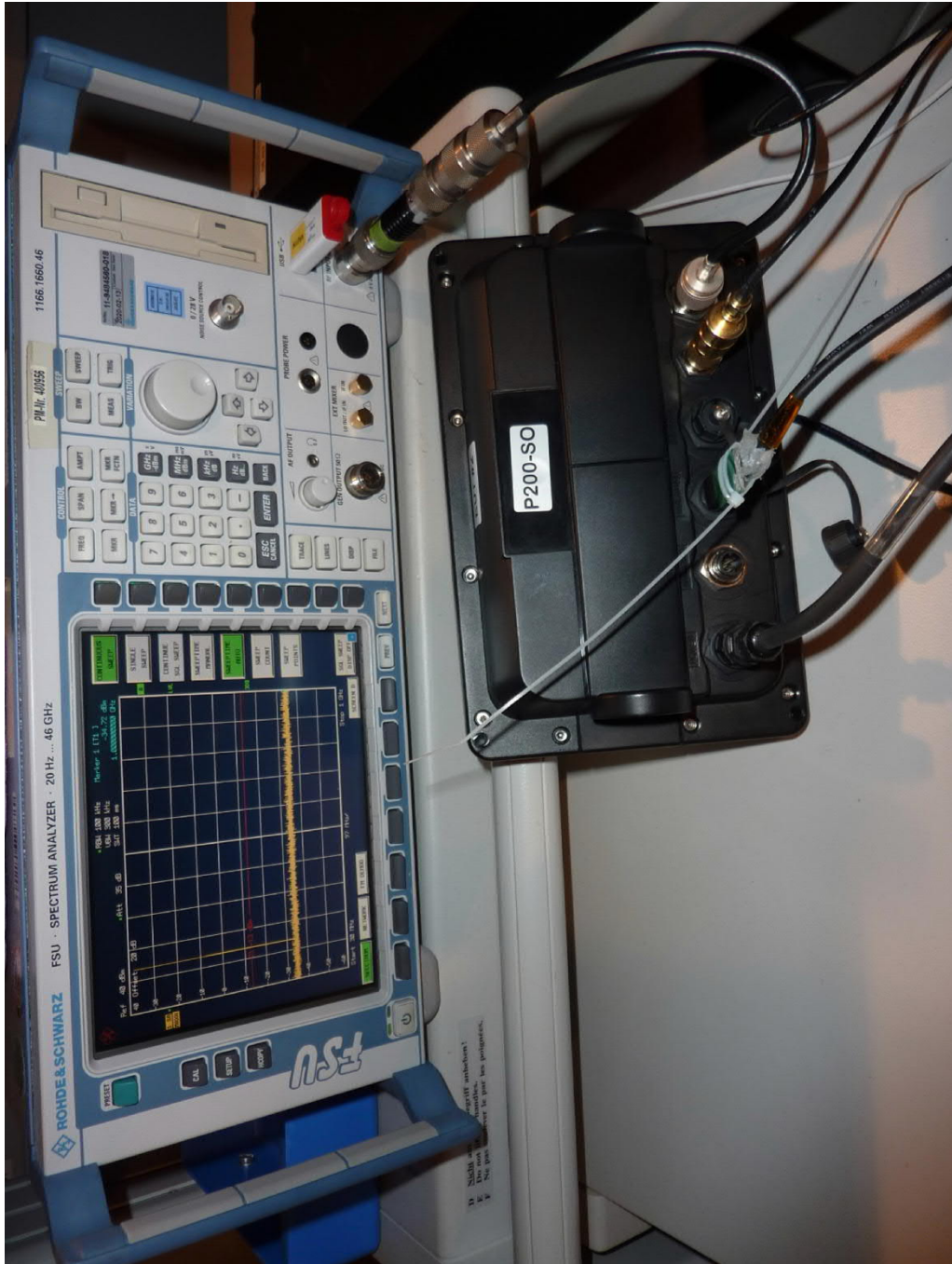
Test setup measurements at antenna port
