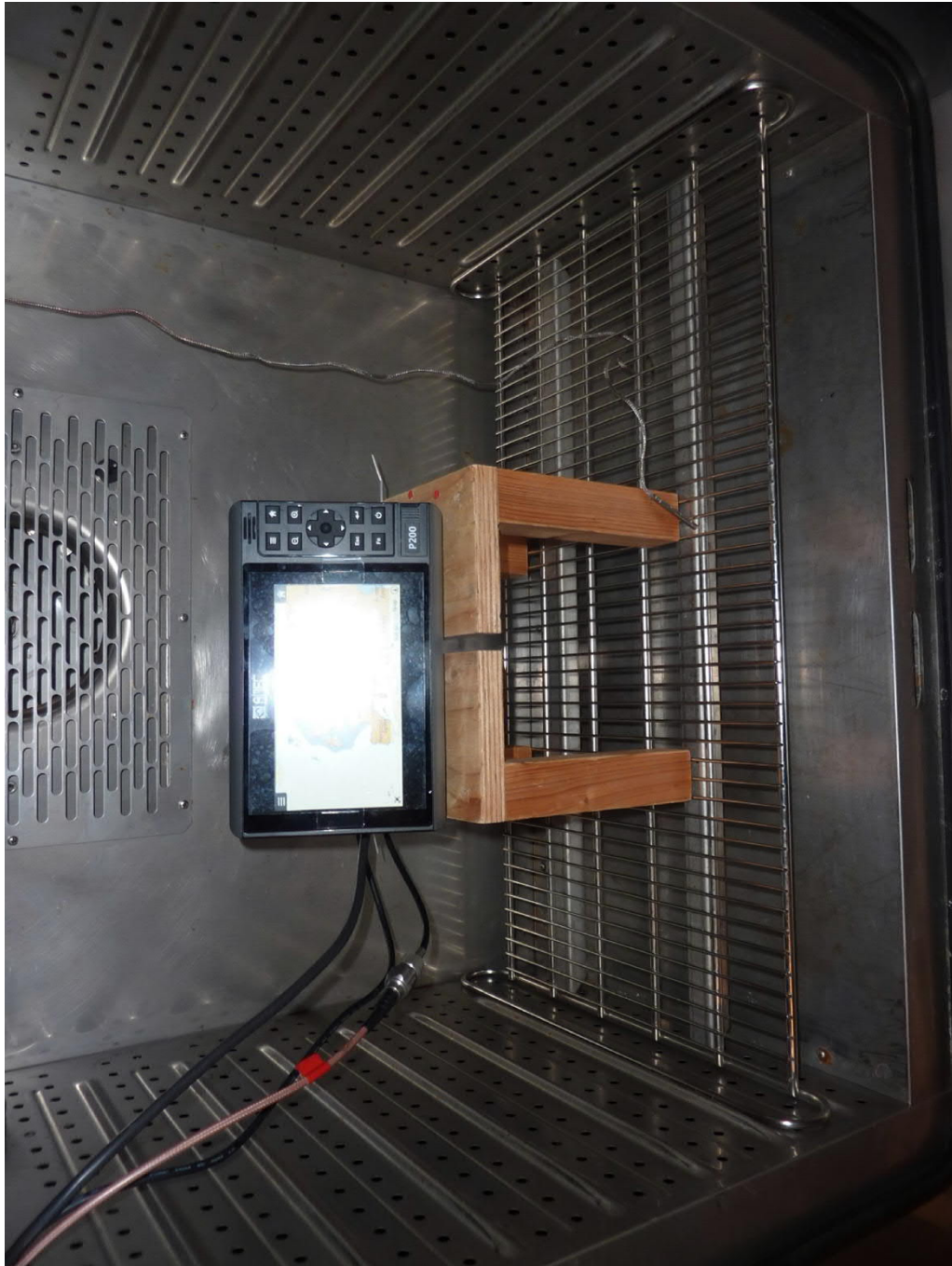
Test setup temperature chamber
