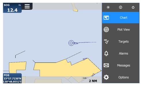
The P200 contains an application which will display AIS targets received, along with its own vessel position on a basic world chart by default. It supports the C-MAP 4D to provide more detailed and high-resolution charts which can be purchased separately by C-MAP dealers. The basic chart operations:
