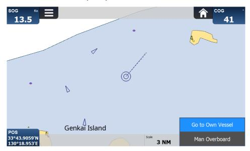
When pressing the Fn Key and select "Man overboard", you can create a Man Overboard (MOB) for an emergency. This means:
