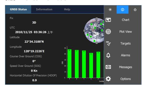
The Device Information can be accessed by pressing on the lower-left corner on chart or plot view where the latitude and longitude are displayed.
