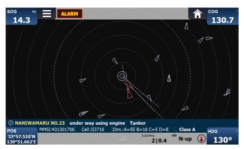
Plot view is the screen to show the location of other AIS targets relative to your own vessel. The own vessel's static data is displayed on the blue bar.
