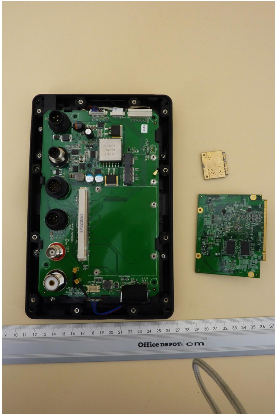
P200-CS, internal view 3 (PCB 1 and 2 removed)
