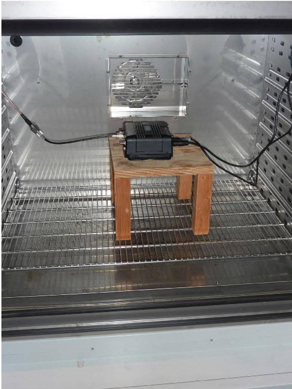
190014_e.jpg: WIDELINK B600S, test setup temperature chamber
