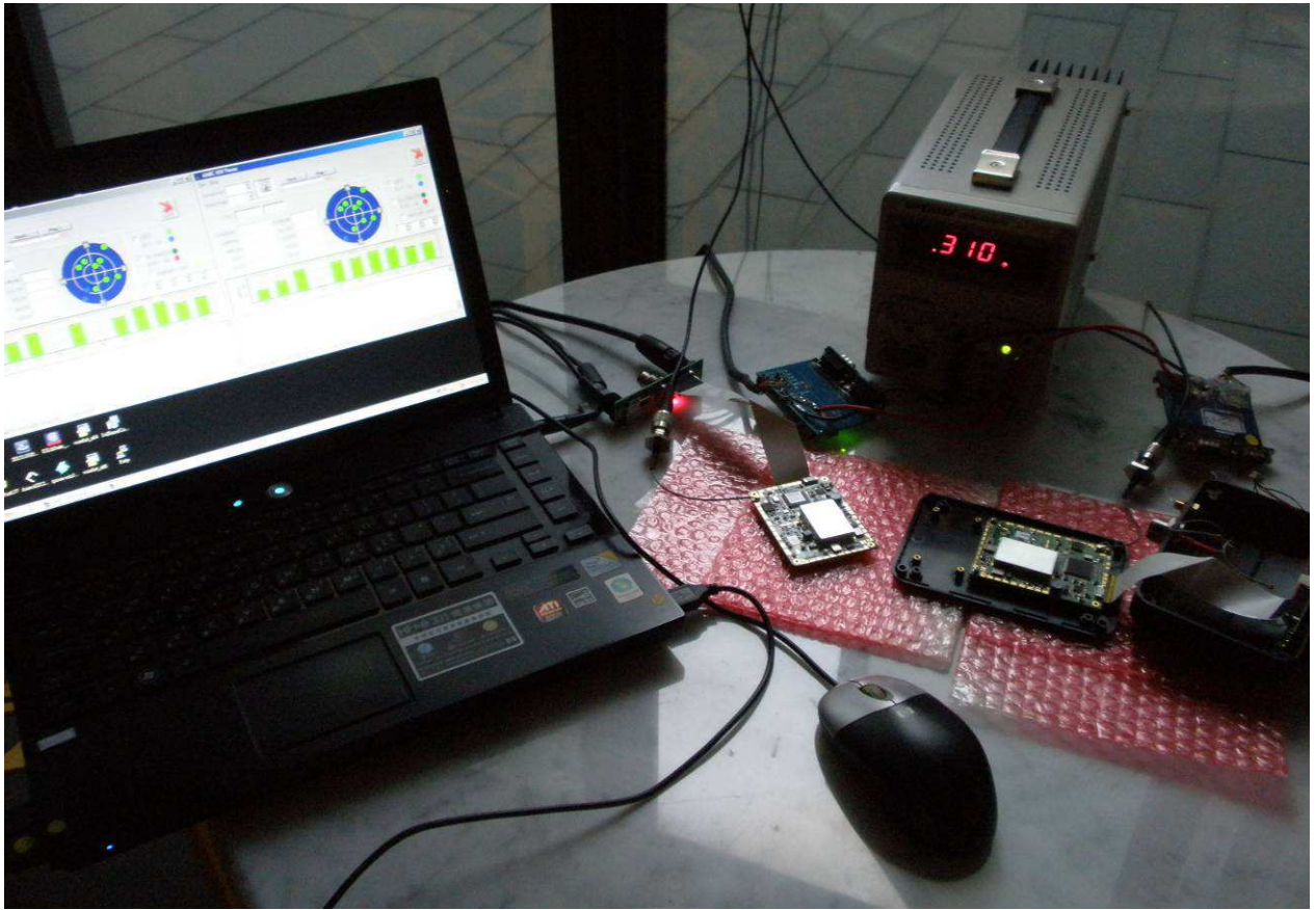
Figure 7 Test Set up for of AMY-6M and EVA-M8M at CAMINO-108
