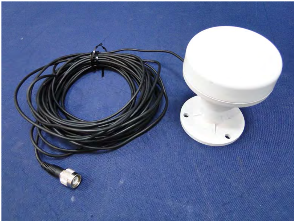
(8) EUT Photo _ GPS antenna with 10m Cable
