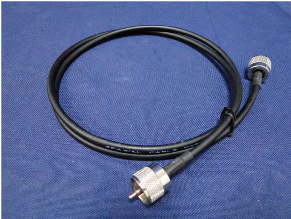
(4) EUT Photo _ VHF Radio Cable
