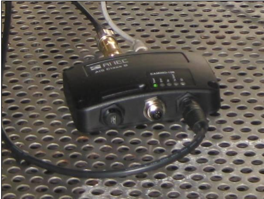
Picture 2: Test set-up EUT in climatic chamber
