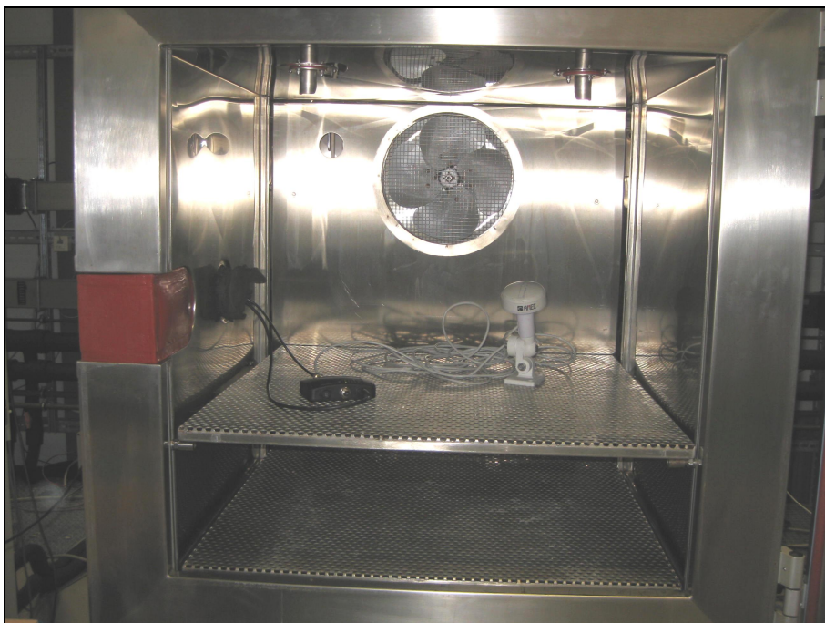
Picture 2: Test set-up EUT in climatic chamber
