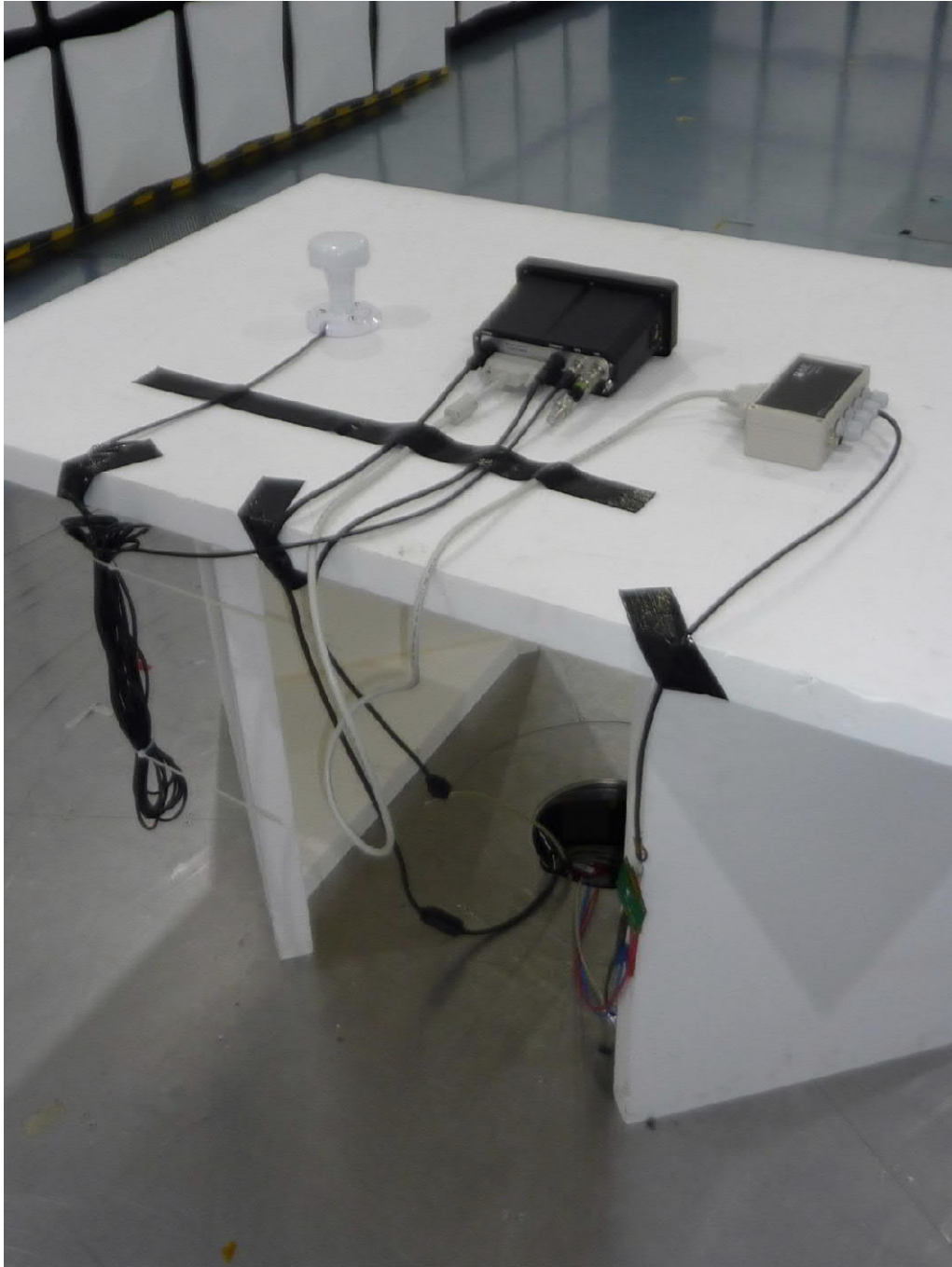
Test setup fully anechoic chamber (below 1 GHz, Pos. 1)
