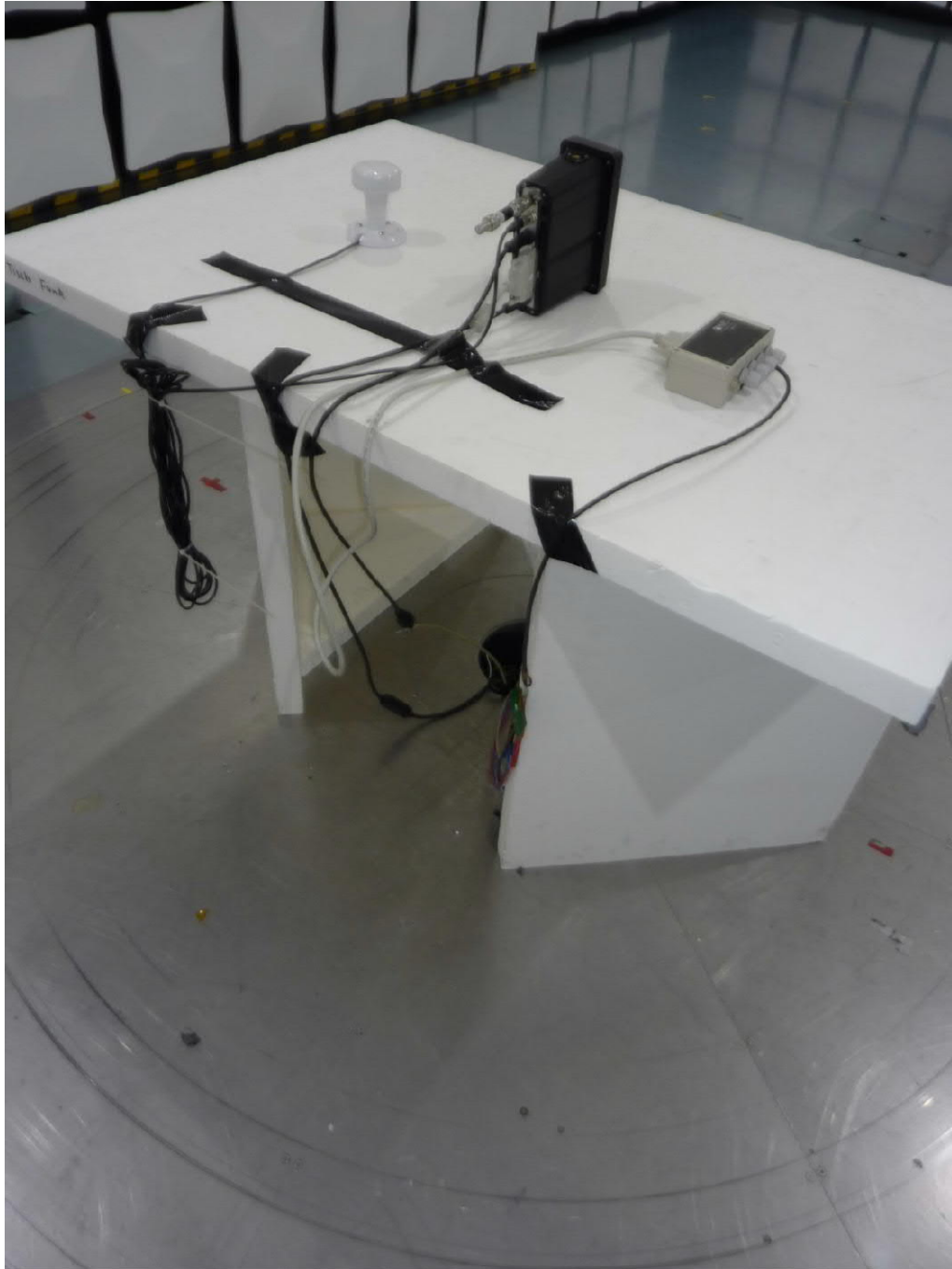
Test setup fully anechoic chamber (below 1 GHz, Pos. 2)
