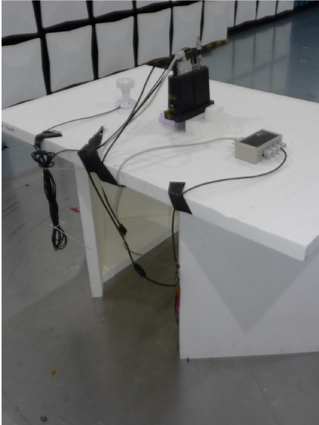
Test setup fully anechoic chamber (below 1 GHz, Pos. 3)
