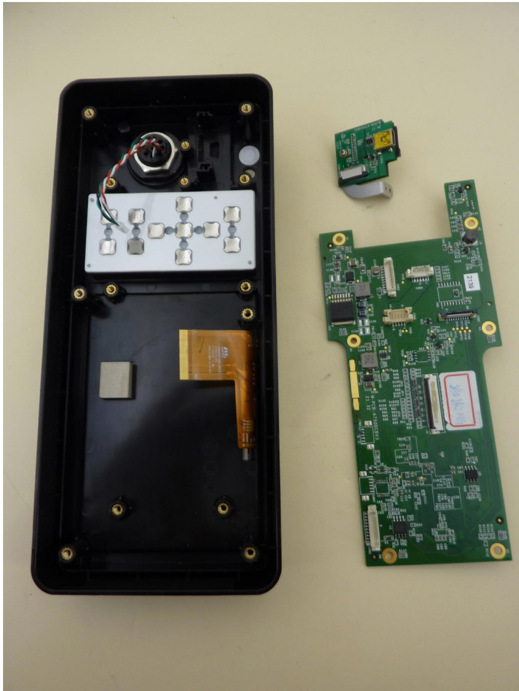
Internal view 4, front cover, PCBs removed
