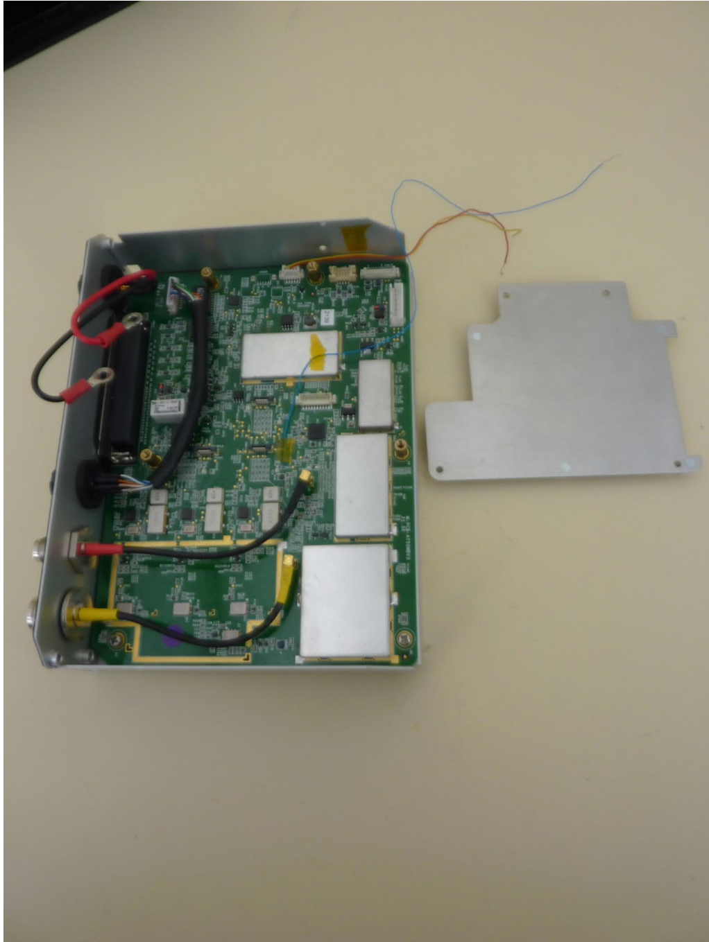
Main part, shielding removed
