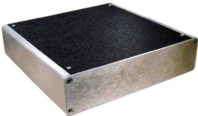
The SkyeTek SR900RCP antenna is a high performance, high efficiency RFID antenna designed to work with the SkyeTek SR100. It features a rugged aluminum case with ABS plastic radome, which houses a Right Hand Circularly Polarized antenna for use in the 902-928MHz spectrum. The antenna has excellent VSWR across the band and small axial ratio to maximize performance with any tag orientation. The antenna is offered with a bulkhead SMA connector.
