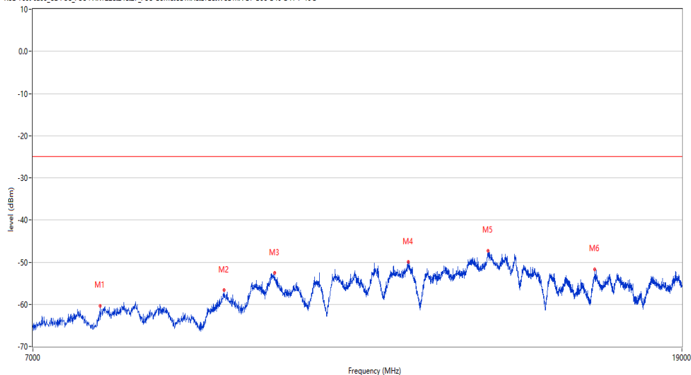
RSE Test case_CE FCC PART22&24&27 FCC GSM&CDMA&LTE&WCDMA B7 B38 B40 B41 7-19G
