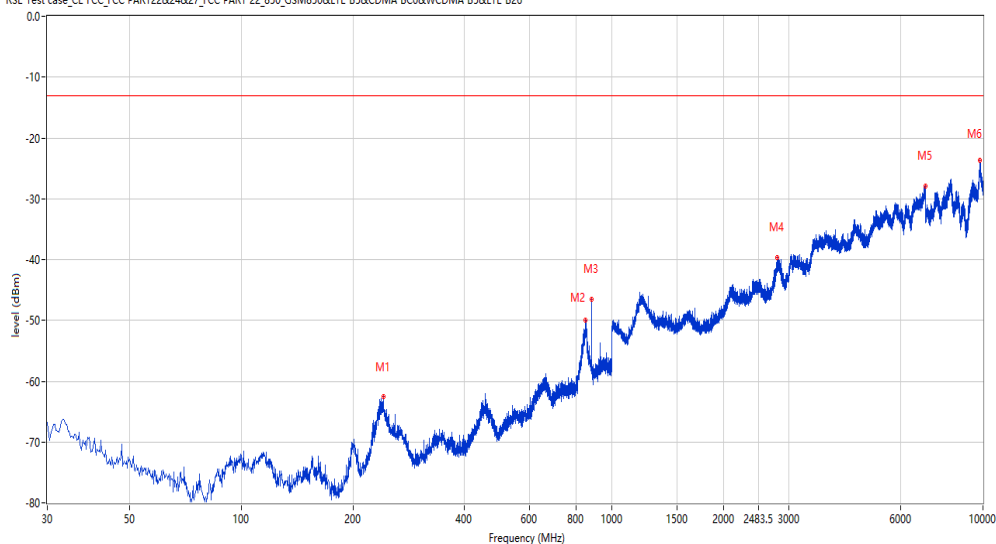
RSE Test case_CE FCC PART22&24&27 FCC PART 22_850_GSM850&LTE B5&CDMA BC0&WCDMA B5&LTE B26
