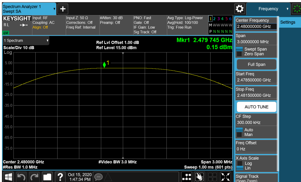
Figure 3: Peak Output Power, 2480MHz
