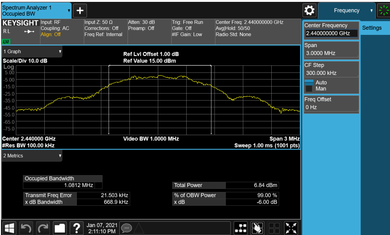
Figure 5: 6dB Bandwidth and 99% Bandwidth, 2440MHz
