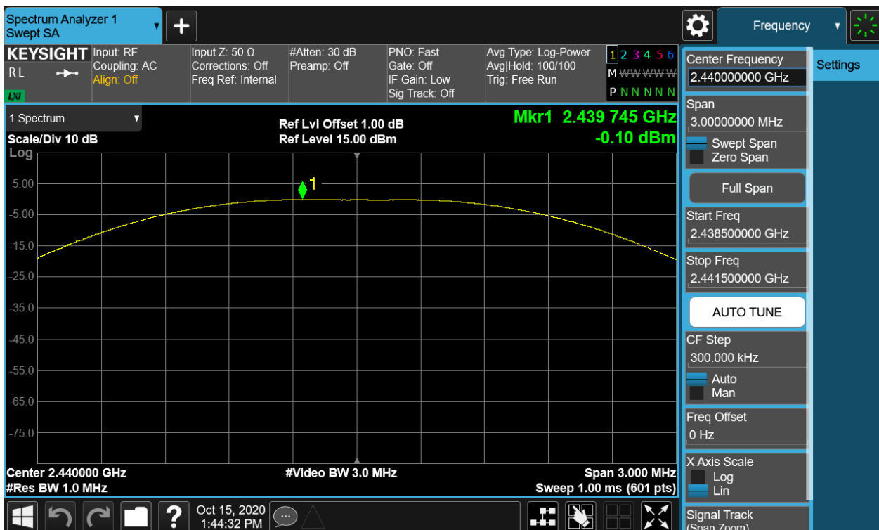
Figure 2: Peak Output Power, 2440MHz
