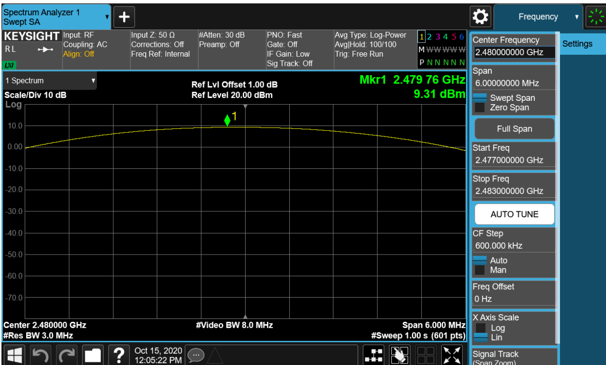
Figure 6: Maximum Conducted Output Power, 2480MHz, \pi/4 -DQPSK
