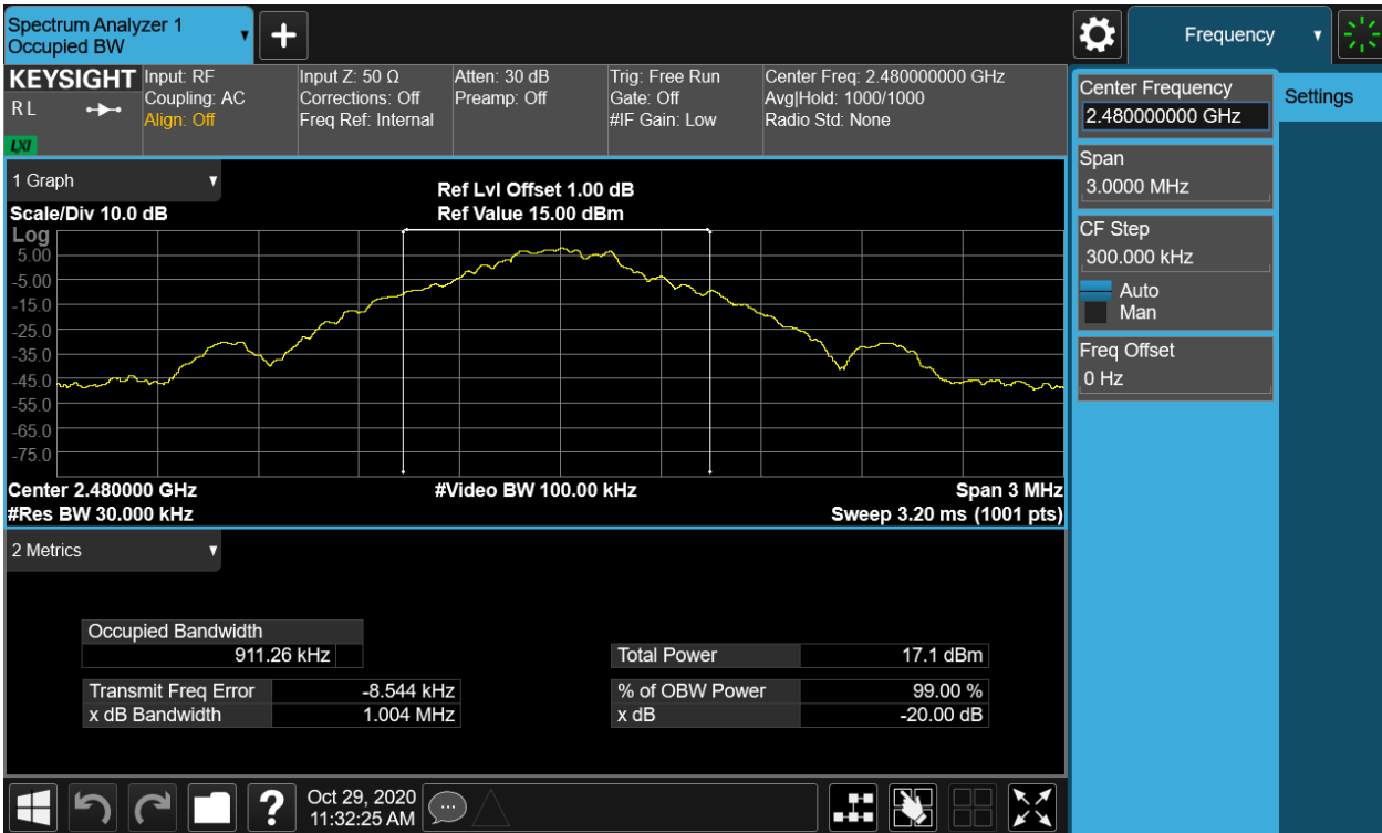
Figure 12: 20dB Bandwidth and 99% Bandwidth, 2480MHz, GFSK
