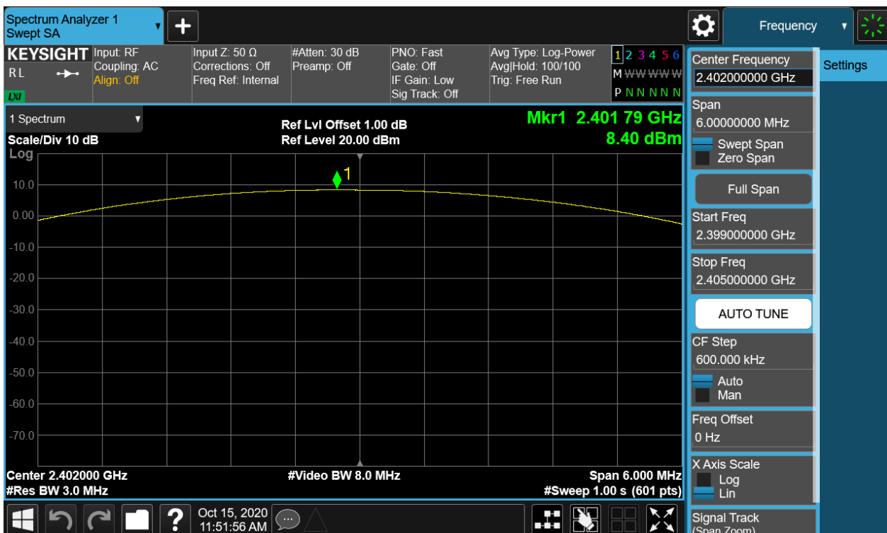
Figure 4: Maximum Conducted Output Power, 2402MHz, \pi/4 -DQPSK
