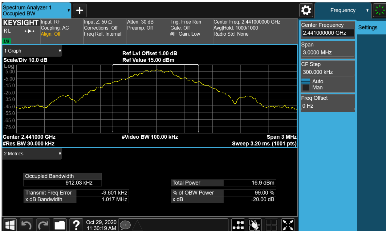
Figure 11: 20dB Bandwidth and 99% Bandwidth, 2441MHz, GFSK
