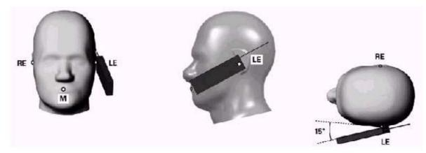
Figure 3 Tilt position of the wireless device on the left side of SAM
