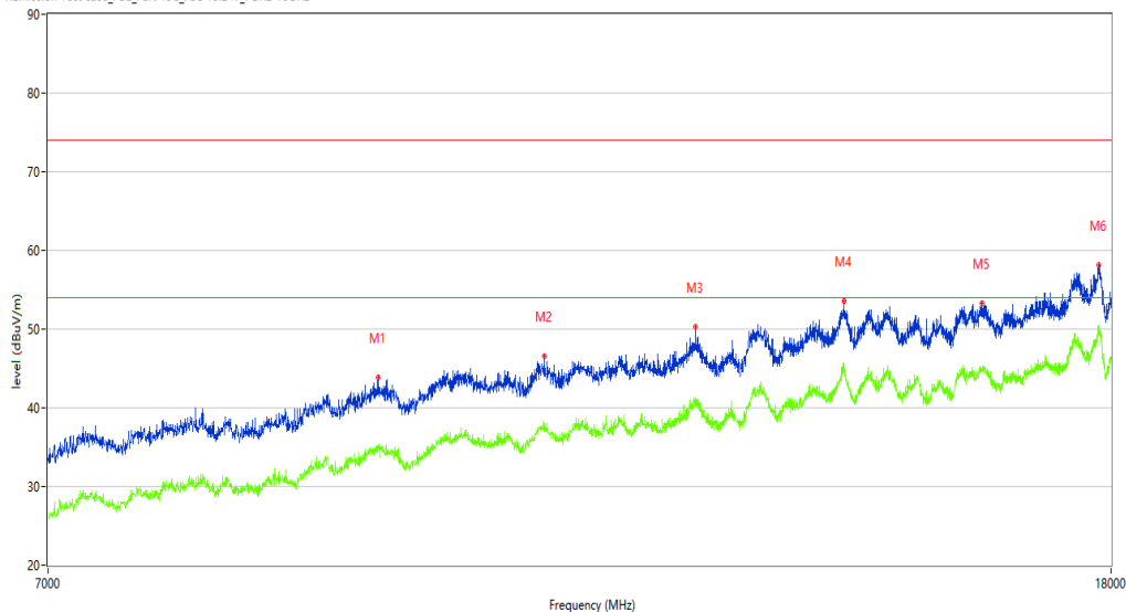
REmission Test case_FCC_Part 15C_FCC 15.247_7GHz-18GHz
