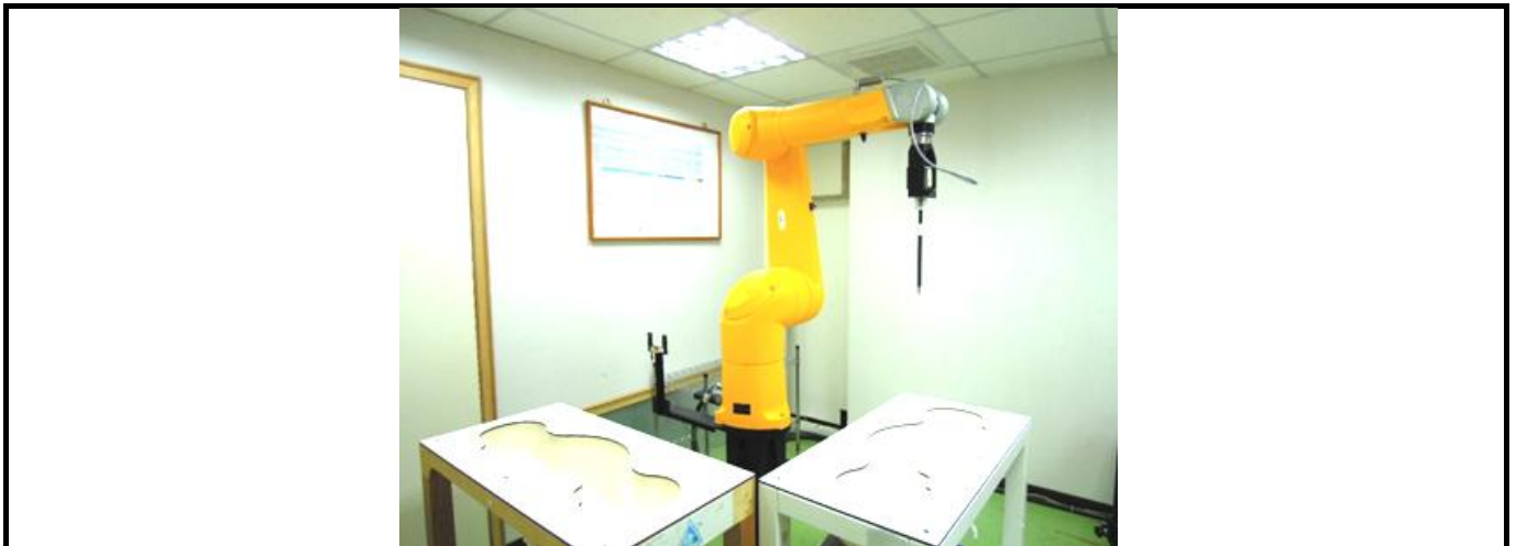
Fig-3.2 DASY5 Measurement System
