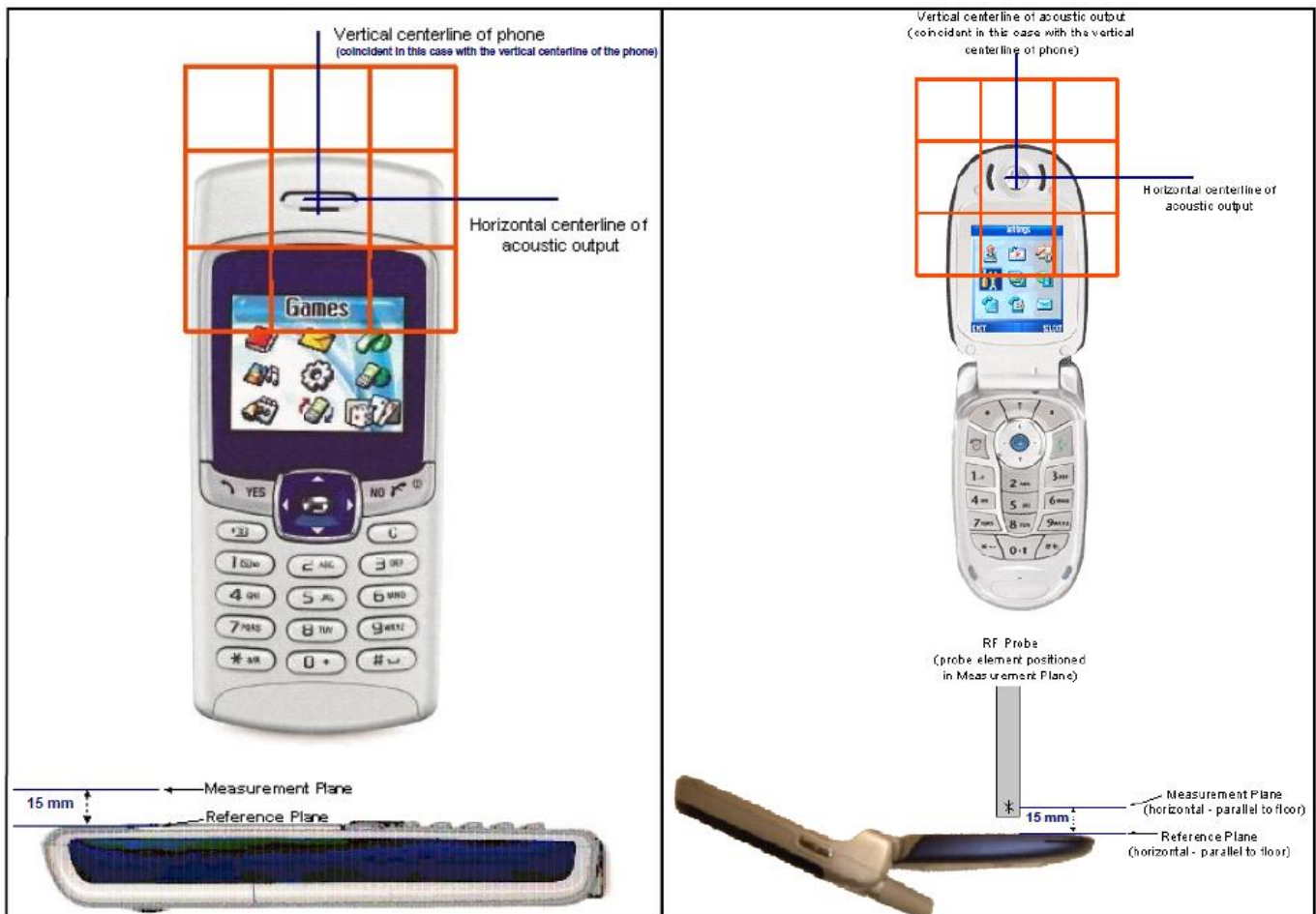
Fig-3.4 EUT Reference and Plane
