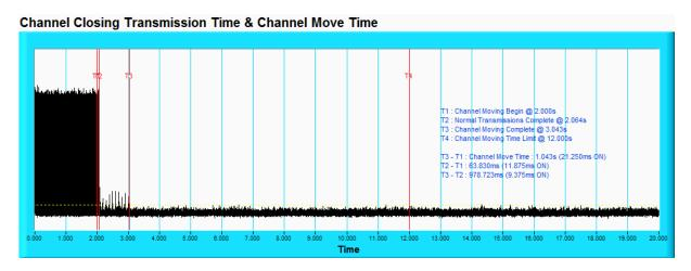
**NOTE**: T1 denotes the start of Channel Move Time upon the end of the last Radar burst. T2 denotes the data transmission time of 200ms from T1. T3 denotes the end of Channel Move Time. T4 denotes the 10 second from T1 to observe the aggregate duration of transmissions.
