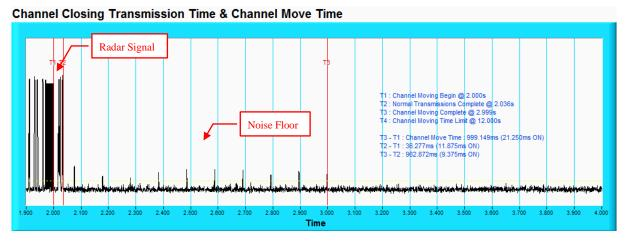
NOTE: Zoom in of the first 2000ms after radar signal applied.
