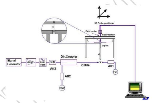
Figure 5 Illustration of system validation test setup
