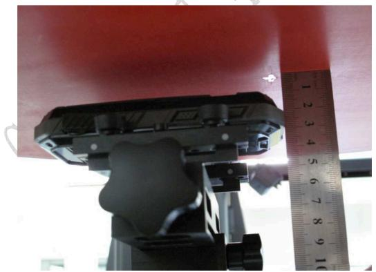
Picture 6: Body SAR Back to the phantom
