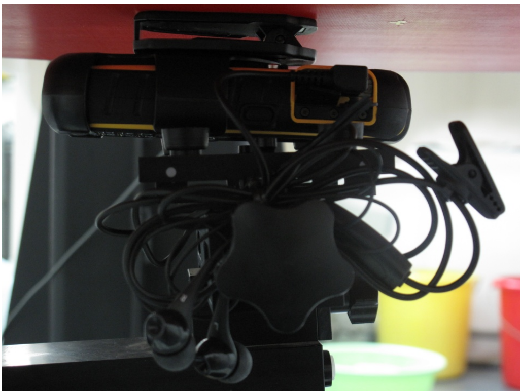
Body SAR with belt and earphone
