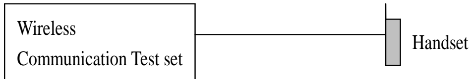
Demonstration of Conducted power measurement
