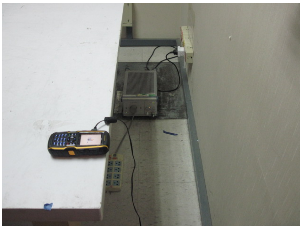
Description: Conducted Emission Test Setup
