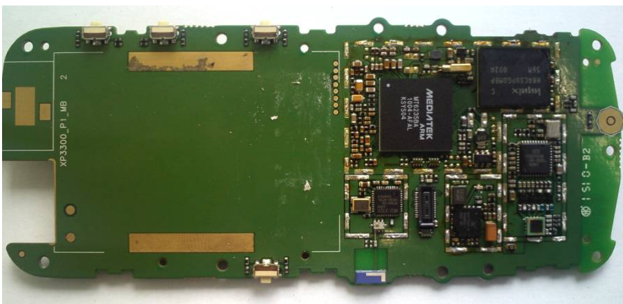
Picture 2: the top view of the PCB with the shielding cover removed
