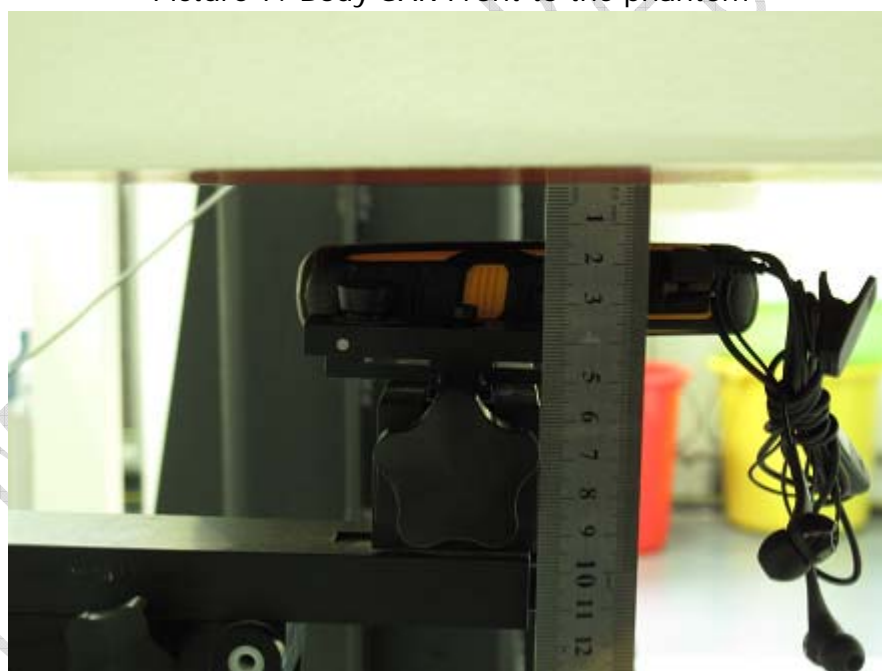
Picture 8: Body SAR Back to the phantom with earphone
