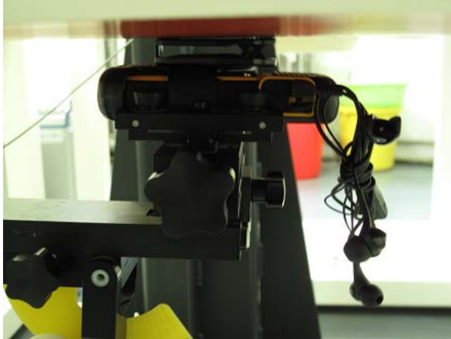
Picture 11: Body SAR Back to the phantom with belt and earphone
