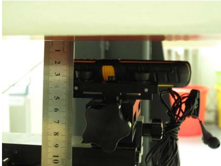
Picture 9: Body SAR Front to the phantom with earphone
