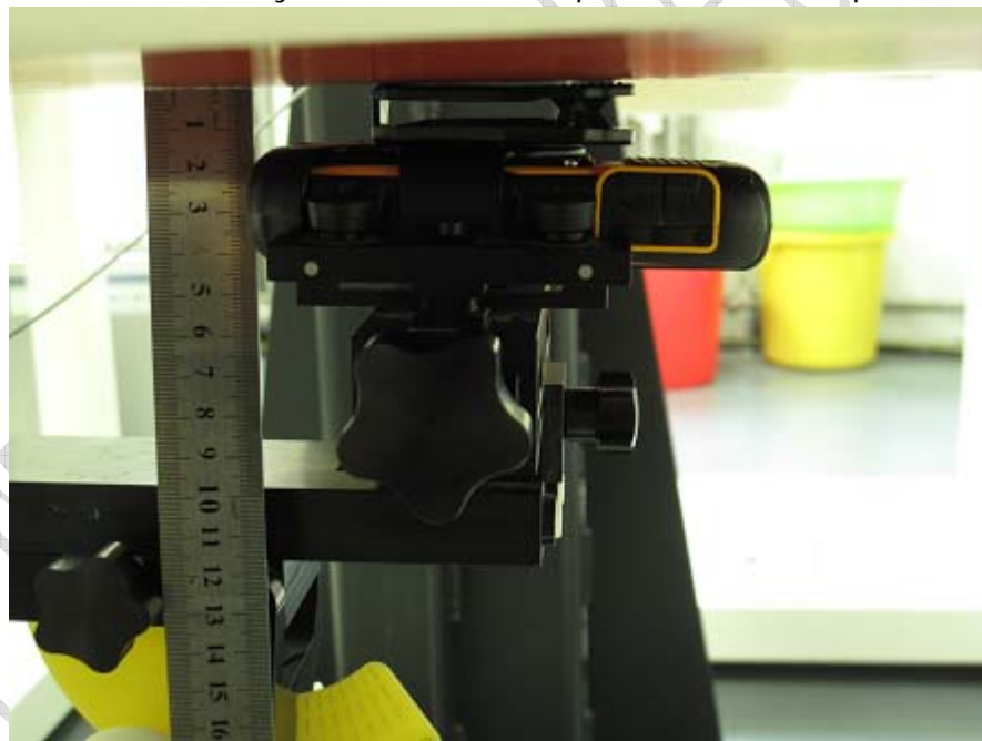
Picture 10: Body SAR Back to the phantom with belt
