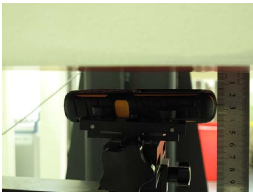
Picture 7: Body SAR Front to the phantom
