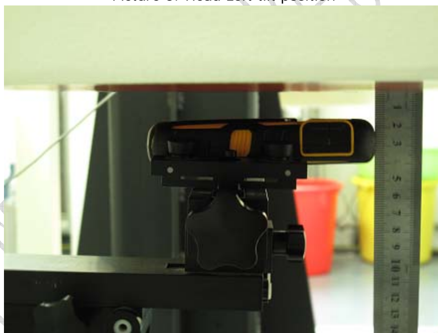
Picture 6: Body SAR Back to the phantom
