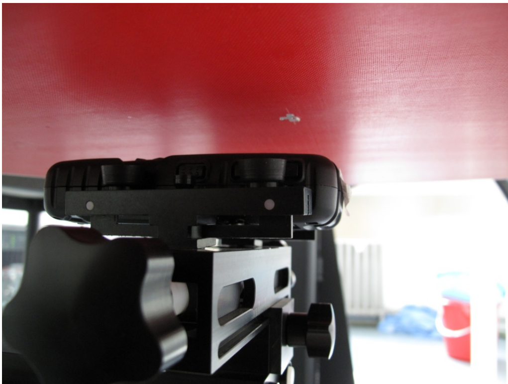
Picture 7: Body SAR Front to the phantom
