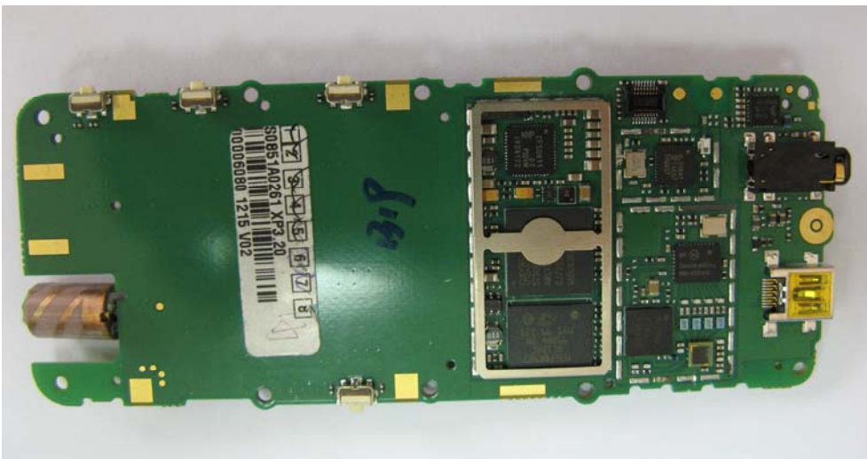
Picture 2: The top view of the PCB with the shielding cover removed
