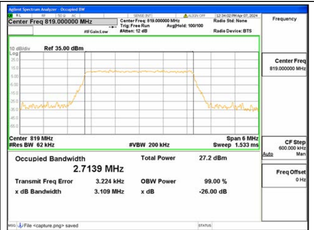
B26 Part90 / 3MHz / 16QAM/ Mid CH
