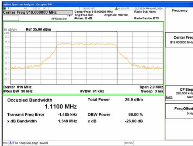
B26 Part90 / 1.4MHz / 16QAM/ Mid CH
