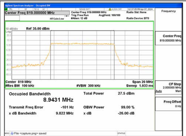
B26 Part90 / 10MHz / 16QAM/ Mid CH
