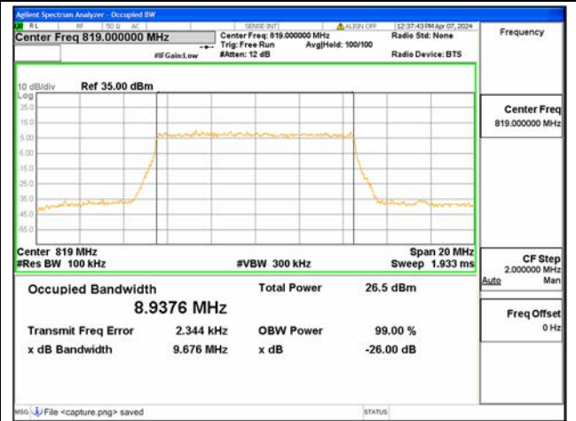
B26 Part90 / 10MHz / 64QAM/ High CH
