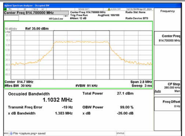
B26 Part90 / 1.4MHz / 16QAM/ Low CH
