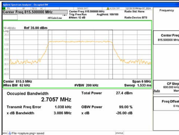
B26 Part90 / 3MHz / 16QAM/ Low CH
