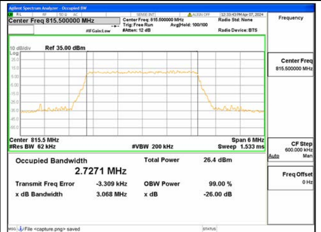
B26 Part90 / 3MHz / 64QAM/ Low CH
